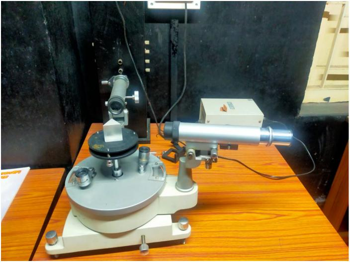
The above instrument is known as Spectrometer. This is help us to determine the angle of prism, refractive index of the material of a prism. Also we can do light related experiment including grating.
