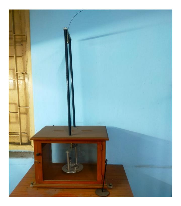
We can calculate the Moment of Inertia of a body about its axis passing through its centre of gravity by using the above instrument.
