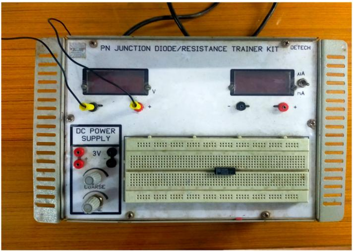
To study the forward and reverse characteristic curve of a semiconductor diode, we use the above instrument.
