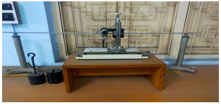
This instrument is use to determine the Young's modulus of a material of the beam by flexture method.
