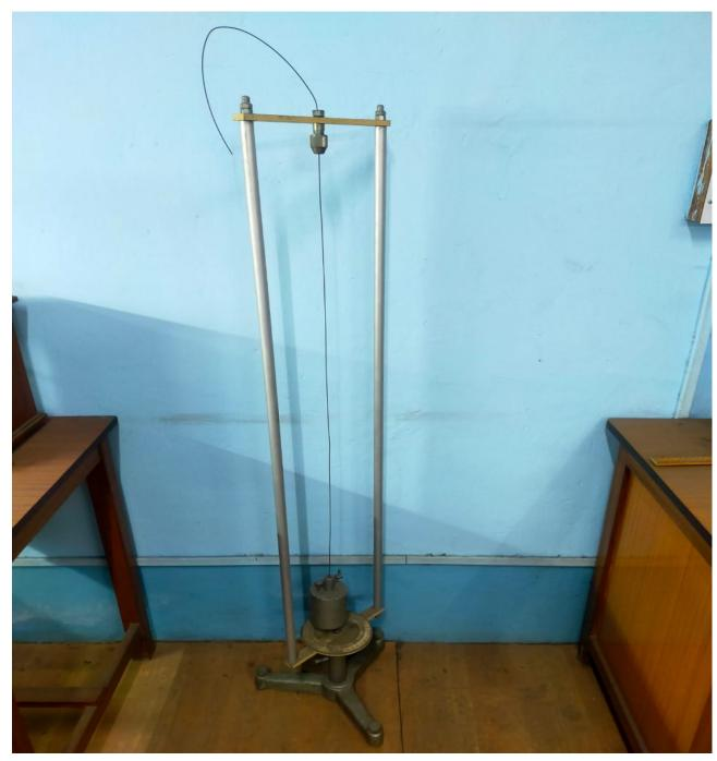
This instrument is use to determine the rigidity modulus of the material of a wire by dynamical method.
