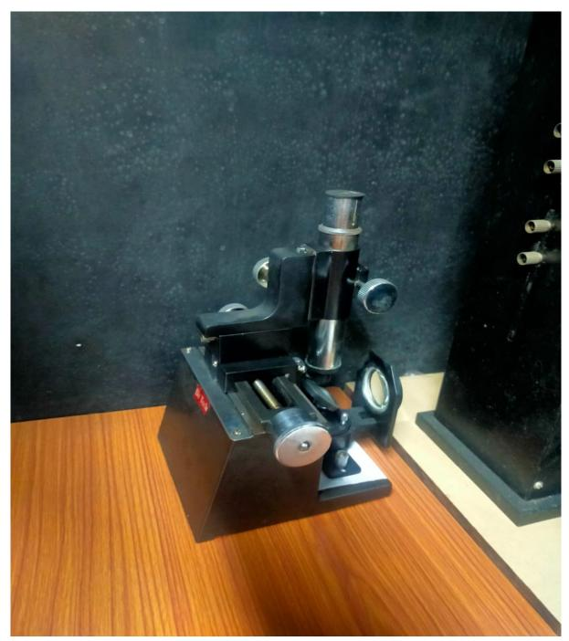
This is help us to calculate the wavelength of a sodium light by Newton's ring method.
